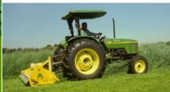
Figure 2. A high-speed flail mower converts the cover crop to a mulch without disturbing the soil.
